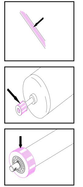
1.Remove the drive belt and check the grooves in belt for dirt or dust and clean it.
